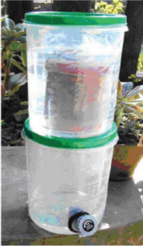
The pottery candle system shown above gives 2.0 to 3.0 liters of filtered water per hour. The system is very effective, acceptable to users and low priced. These can be made almost anywhere, using local resources.
